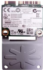
Position the WiFi module and the "mini half bracket" exactly as shown.
