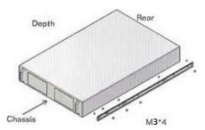
**STEP 5.** Attach the inner slide member to your chassis using M3\*4 screw from screw kit.
