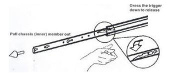
**STEP 1.** Take the inner member (Bin Yuann slide) apart by pulling the front, activating the release latch forward.
